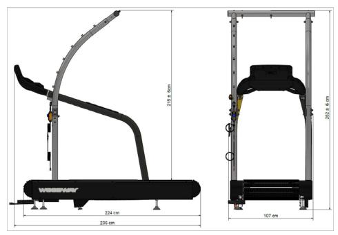
Fig. 6 Dimensions, Fall Protection System for Pro XL Treadmill
