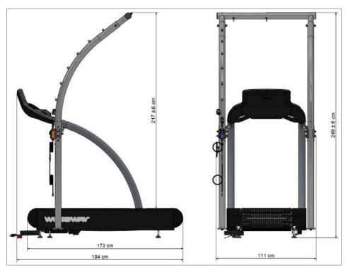
Fig. 4 Dimensions, Fall Protection System for 4Front Treadmill
