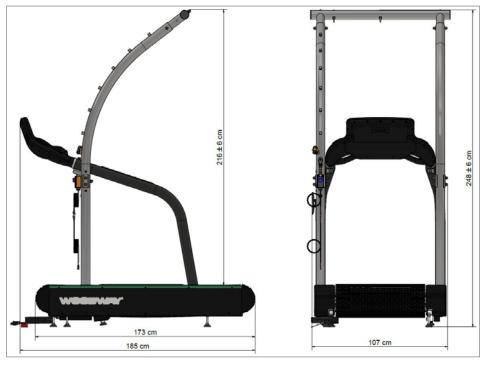
Fig. 5 Dimensions, Fall Protection System for Pro Treadmill
