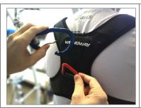
Before training, the user's mounting ring is hooked into the fall protection system snap link.
