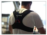
Ensure that the safety line is not twisted and the snap link hook is securely locked.
