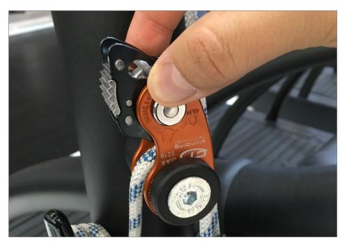
Fig. 9 Rope lock, Locking Pawl Open
