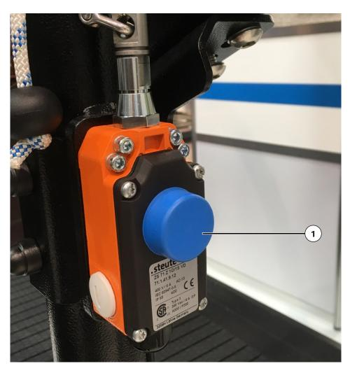
Fig. 12 Pull Switch with Release Button
